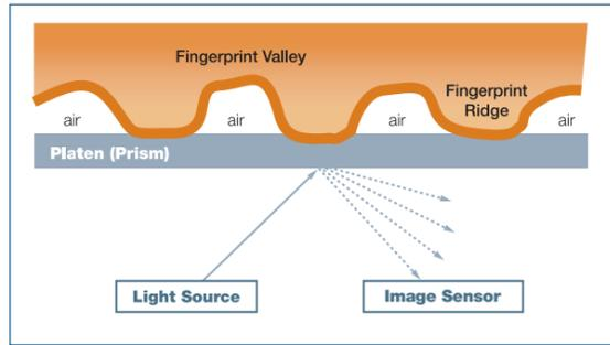
Figure 3: Optical principle of Frustrated Total Internal Reflection
